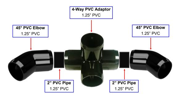
PVC Light Head Assembly can either be glued together using PVC glue or it can be assembled using #6 x 3/8" stainless steel screws which allows the 45° Elbows to be adjusted or changed if need be.
